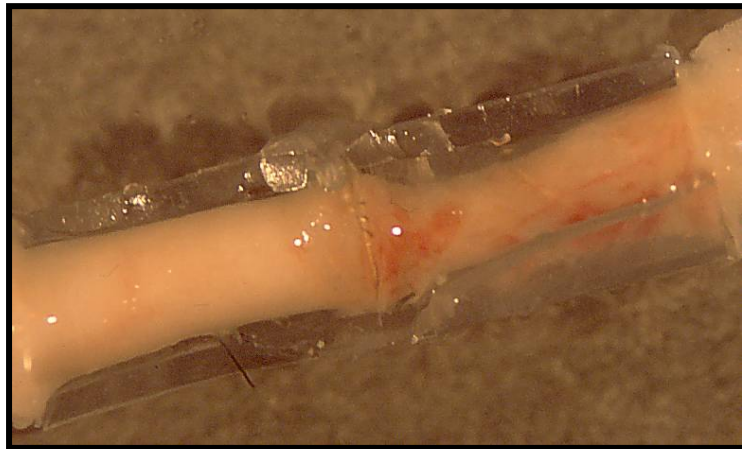
Nerve regenerated through the regenerative electrode
